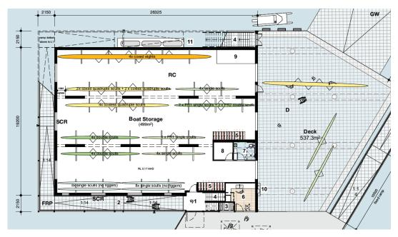
The boat storage area shall incorporate roller or panel lift doors for ease of access to the rowing sculls and an independent pedestrian access door, which also facilitates access to the ramp to the upper level. This ramp shall provide 1800 minimum clear width between handrails and provide level rest landings at intervals not exceeding 9 metres in accordance with AS1428.1 to satisfy clauses D4D3 and D4D4 of the BCA and DDA Premises Standards.
